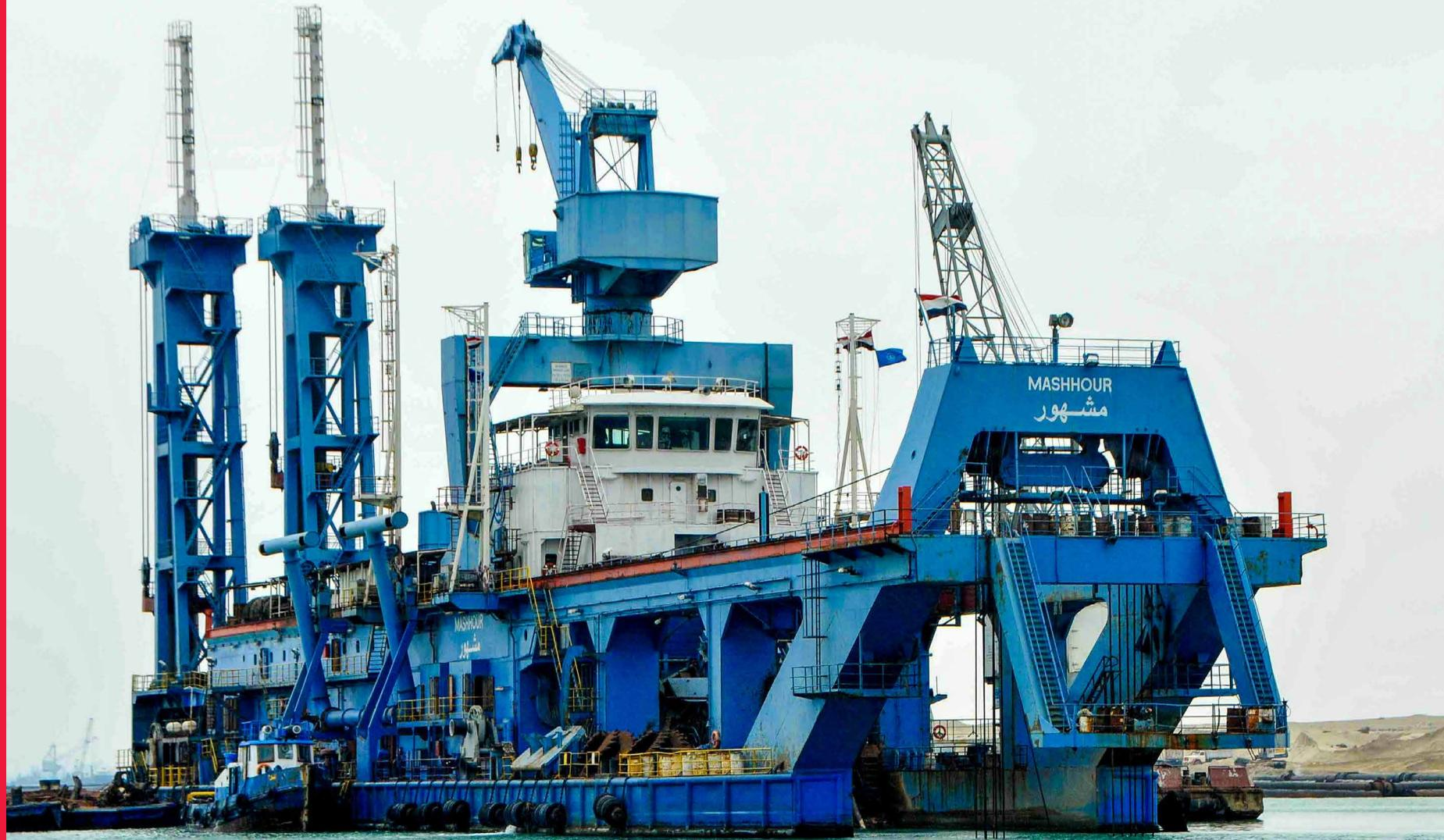
*Dredger (Mashhour), on duty dredging the new suez canal. it is the largest cutter suction dredger in the sca dredger fleet.*
